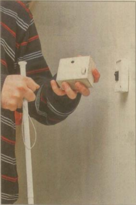
■ The parts of Roshni: the wall sensor (right) and the wearable device (centre)
